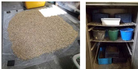
Figure 6.3. Left: Spread pea gravel for natural ventilation. Right: Fine sand dried in the furnace.
